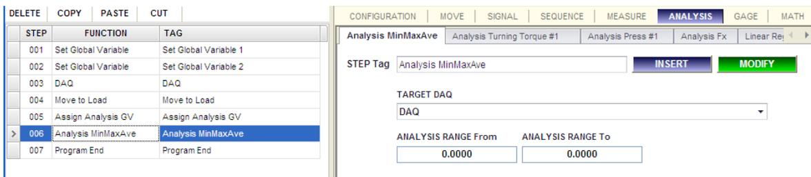
You added “Assign Analysis GV” just before above “Analysis MinMaxAve” step. And select the “Analysis MinMaxAve” as Target Analysis. When you select the Target Analysis, you can see the Global Variable for Parameters Name Tags are changed to proper name. And by assigning “Global Variable #1” and “Global Variable #2” as the analysis range of the Target Analysis step, the “Analysis MinMaxAve” step will analyze within 10 to 50.
