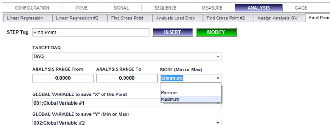
1. **Description:** It returns the Minimum(or Maximum) point (x, y) in the selected target DAQ curve. You can also define your analysis range of the target DAQ.
