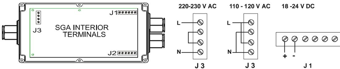
Standard mains 2 or 3 core cable PVC sheathed (unshielded) cable will suffice for the power.
