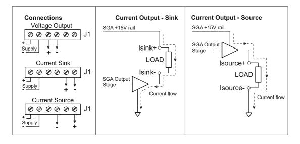
In 'Sink' mode the +ve end of the load is connected to the internal +15V supply on the SGA and the -ve end is connected to the SGA output. The current through the load is 'sunk' by the SGA towards ground (0V). N.B. In this mode neither connection to the output load is electrically common to the load cell. Select this option by fitting the two jumpers, JP1 and JP2 to the 'outside' positions (See Figure 3.2)
