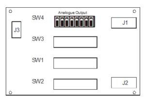
Use switch 4 to select the required output and, if required, the low pass filter and 5V Excitation. (See Tables 3.1 and 3.2)
