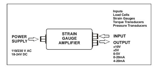
Transducer SENSITIVITY of between 0.1 mV/V and 30 mV/V are possible.
